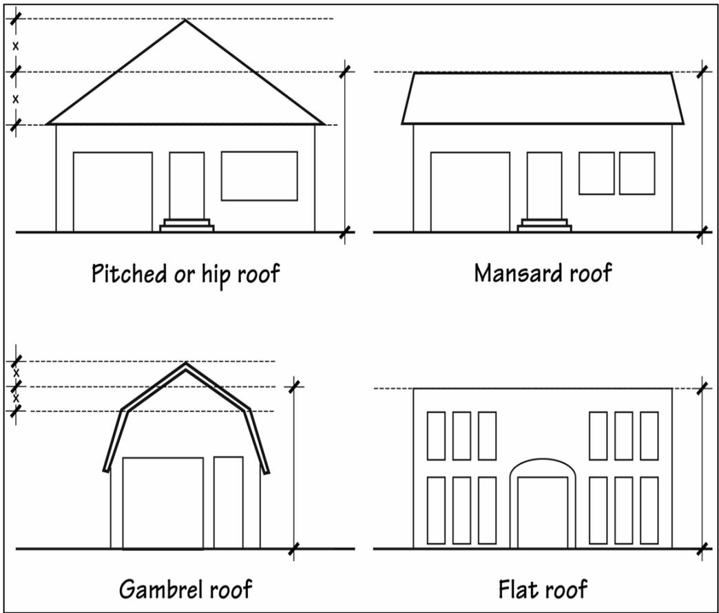
**FIGURE 22-1. Measure building height by roof types.**
