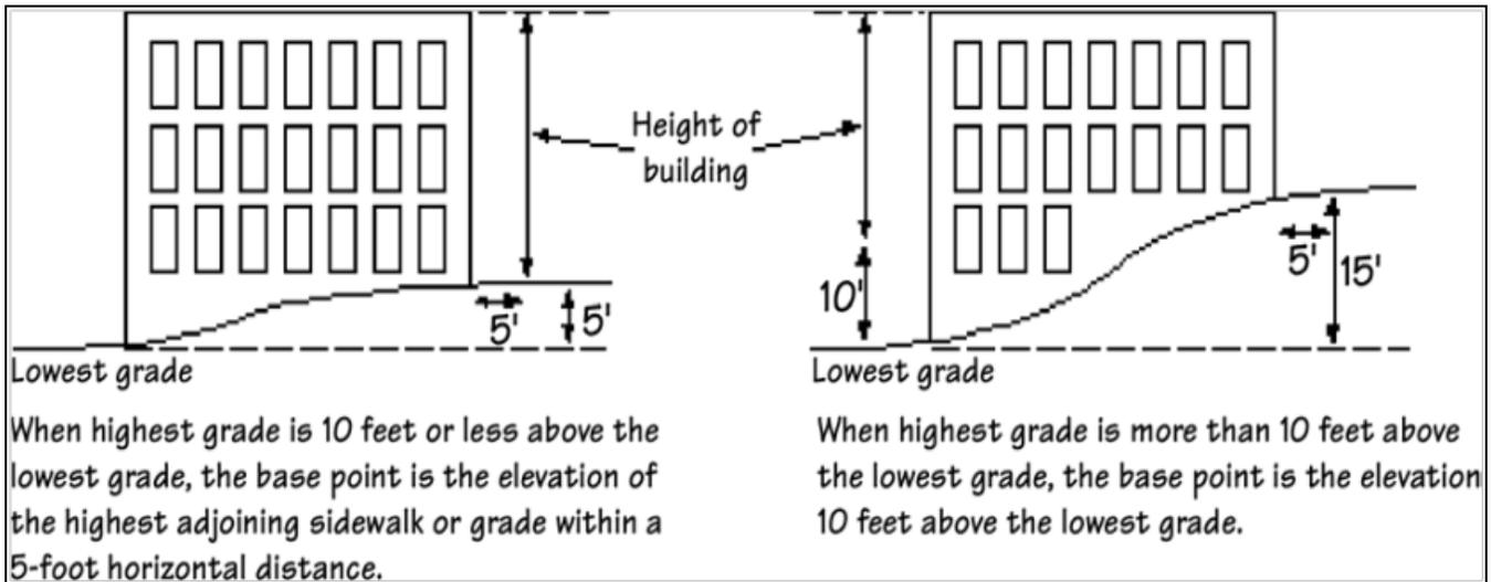
**FIGURE 22-2. Measuring the height of buildings that have a portion below grade.**
